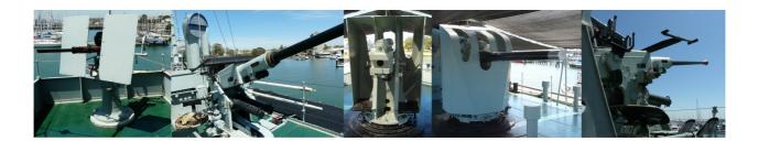
The 4" Deck Gun was manned by a crew of 5 men and was the ships' primary armament, firing a range of specifically tailored shells for different targets.
