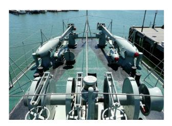
The minesweeping array mounted on the stern was used to undertake the ships' primary purpose; cutting the tethering cables of mines so they could be destroyed with rifle fire. Mines were an insidious threat to the ships of the era, destroying any ship which contacted them, be it enemy, friendly or non combatant.
