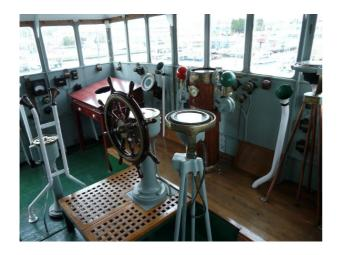
The Bridge was where the ship was commanded from. It housed the ships wheel, ASDIC (early type of sonar) and was crewed by 6 men at all times. The wheelhouse also contained a cluster of voicepipes which carried messages to the various compartments of the ship.
